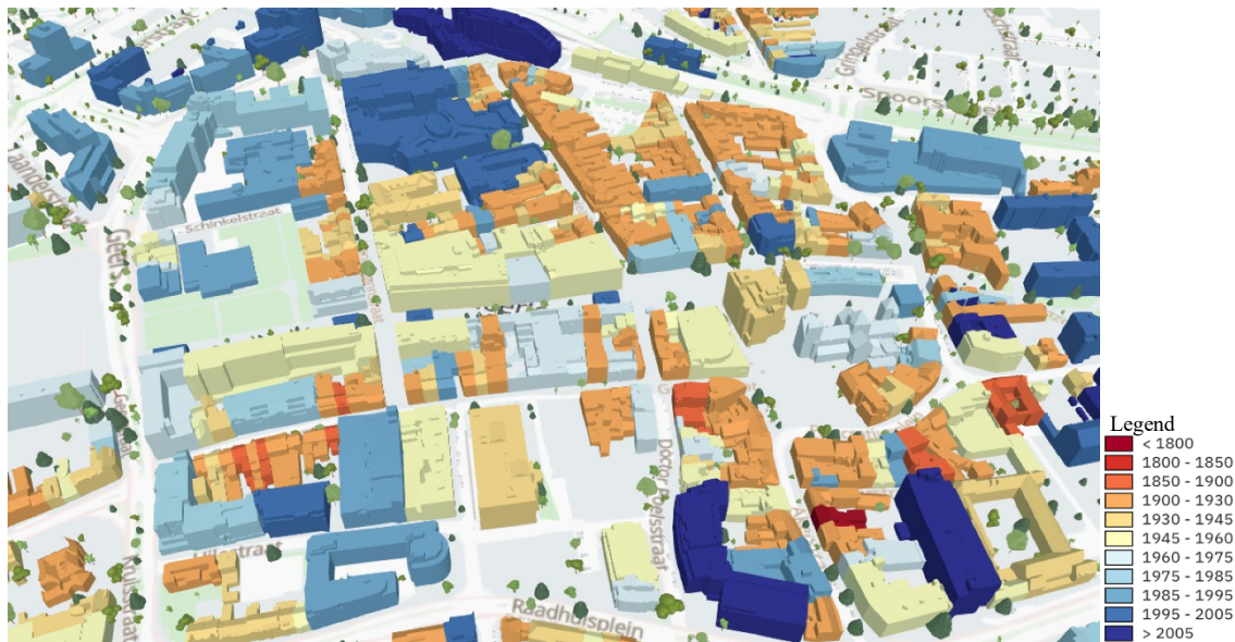
Figure 23 - Prototype digital twin of Heerlen for Age of Buildings at Micro Scale
